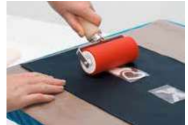
6 After the application is finished use a pressing cloth or a rubber roller to apply additional pressure to the product.
