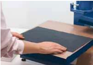
4 Place the carrier material with the motifs facing down in a heat press.
