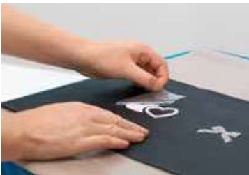
7 Once the product is at least hand warm the transparent film can be removed at an acute angle. The application is now finished.
